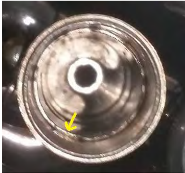
One of the casing slots is indicated by the arrow. There is a second one, directly across the casing, but it doesn't show in this photo.
