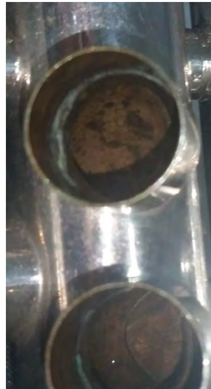
Valve down – holes aligned. (Looks like it needs cleaning!)
